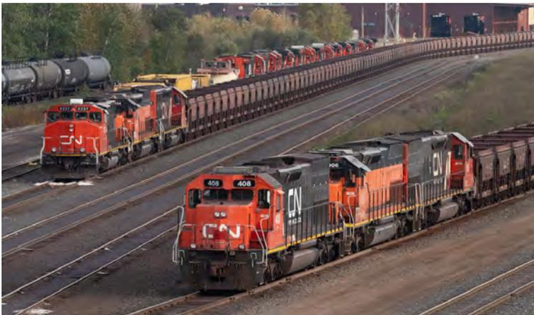
While CN has some of the newest locomotives in North America, it also has the distinction of operating the oldest locomotives on a Class I, with a number of GP 9's still in service. Called GP9 RM's on CN, these relics from the 1950's were completely remanufactured between 1985 and 1994 and have continued to serve CN well into the 21st century.
