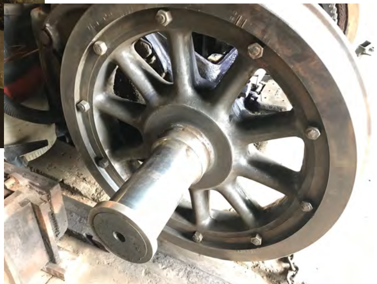
Same wheel after tedious chipping layers off with needle gun and finishing with a wire wheel.
