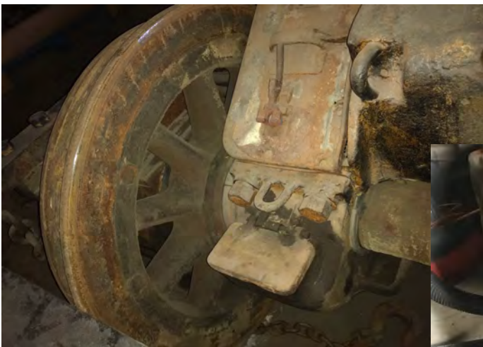
#1 traction motor along with wheel as she was left in the late 60s with layered up crud and rust.
