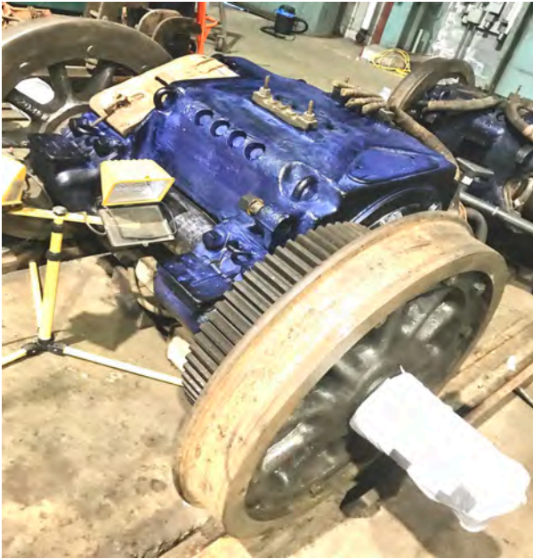
#2 traction motor on home stretch with cleaning, de-rusting and protective paint application.
