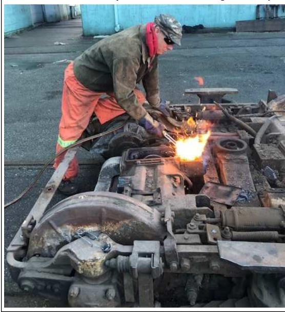
The goal was to make the car a bit lighter, to aid with floor loadings at the new location, so the motors were removed as was the brake rigging.
