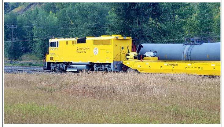
It powers train MW9507-10 which consists of nine cars (three sets of new articulated well cars with rails mounted to accommodate a John Deere excavator that travels as part of the train, and a control cab on the other end so the train is fully bi-directional. The entire train is painted bright yellow. Two additional GP38AC's, numbers 3005 and 3007 are also being converted. (SDHSE)
