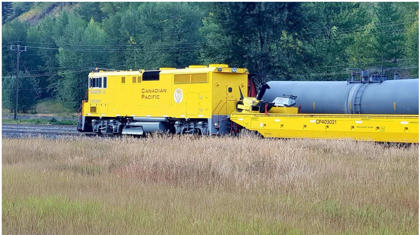
It powers train MW9507-10 which consists of nine cars (three sets of new articulated well cars with rails mounted to accommodate a John Deere excavator that travels as part of the train, and a control cab on the other end so the train is fully bi-directional. The entire train is painted bright yellow. Two additional GP38AC's, numbers 3005 and 3007 are also being converted. (SDHSE)
